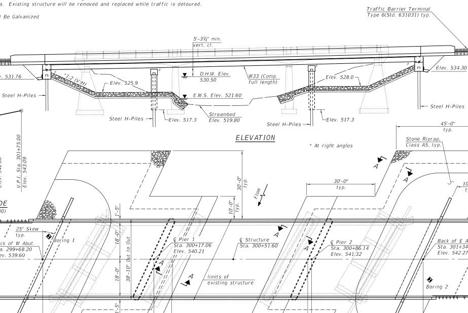
(Along & U.S. Rte. 40) 25° Skew typ. Back of W Abut. Sta. 299+68.20 Elev. 539.60 ¥-<u>30'-0" Bridge approach</u> slab typ. 45'-0" & varies Channel width ₹  $\checkmark$ 69'-1" 48'-10<sup>1</sup>/<sub>4</sub>"  $48' - 10^{1}/_{4}''$ 166'-9½" Back to Back Abutments PLAN DESIGNED JUSTIN T. BELUE STATE OF ILLINOIS CHECKED JOSUE D. ORTIZ-VARELA **DEPARTMENT OF TRANSPORTATION** DRAWN - GLENN W. STOVER 9/23/2020 - 10:31:08 AM CHECKED - RICHARD J. CHAPUT
