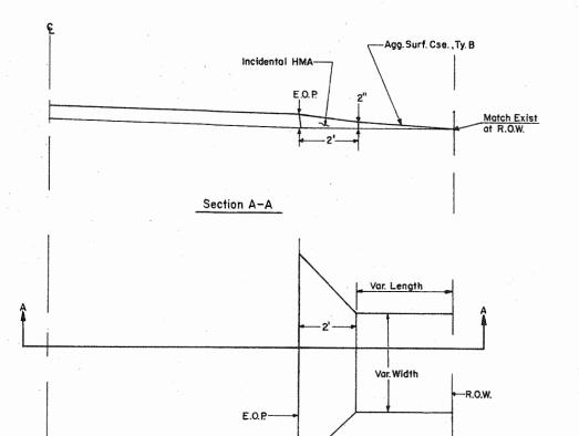
Field Entrance 2' Wedge HMA Surf. Agg. Surf. Cse. (Tons) Ty. B (Tons) O/S Width Station 33+12 LT 20 2 3.0
