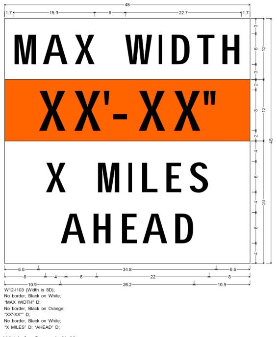
Max Width for Stage I: 9'-6" Max Width for Stage II: 11'-6"
