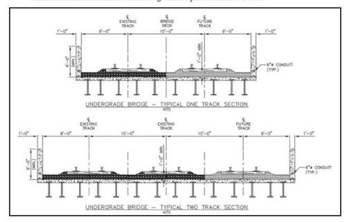
• Minimum horizontal clearance on the bridge shall be provided as shown below.
