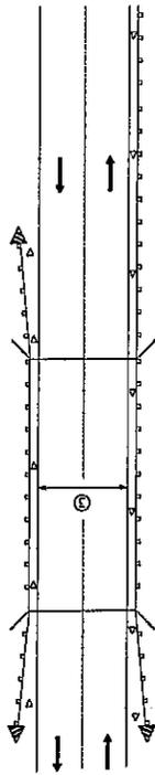
② Bidirectional silver/silver should be used in lieu of monodirectional silver on both sides of two-lane bridges where the bridge pavement is less than 24 (10) wider than the pavement approaching the bridge.
