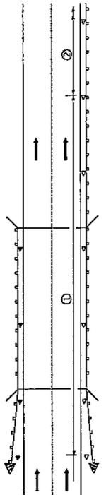
① Spacing 80 ft. (24 m) max. for first 400 ft. (122 m) or curve spacing shown in Standard 63500, whichever is less (min. 4 reflectors regardless of length).
