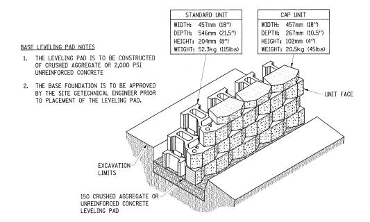
STANDARD UNIT/BASE PAD ISOMETRIC SECTION VIEW
