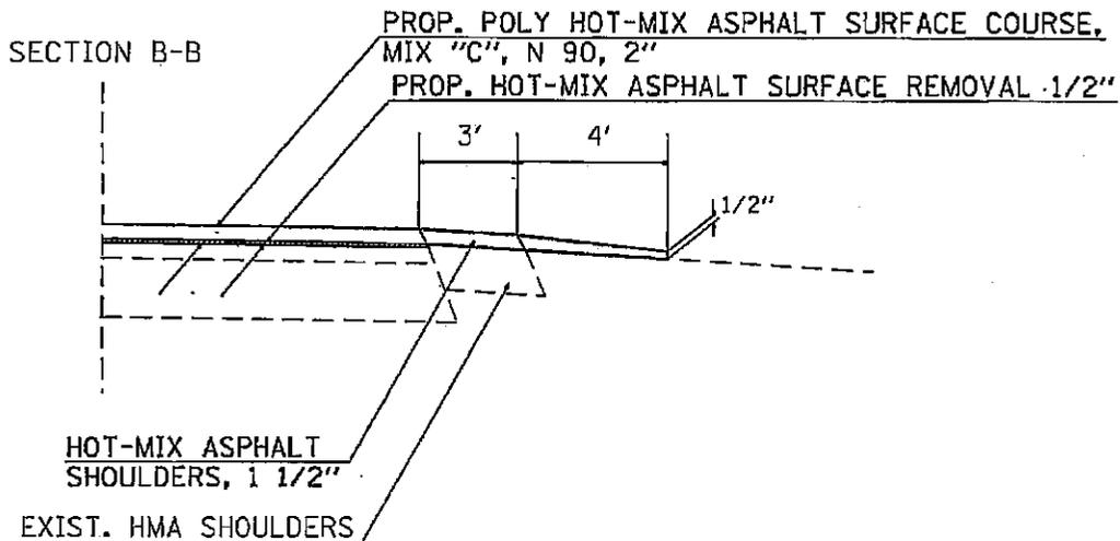
PREPARATION OF EXISTING SURFACE AND ANY EXCAVATION FOR ENTRANCES SHALL BE IN ACCORDANCE WITH ARTICLE 406.19 OF THE STANDARD OF SPECIFICATIONS.
