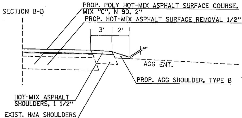
PREPARATION OF EXISTING SURFACE AND ANY EXCAVATION FOR ENTRANCES SHALL BE IN ACCORDANCE WITH ARTICLE 406.19 OF THE STANDARD SPECIFICATIONS.
