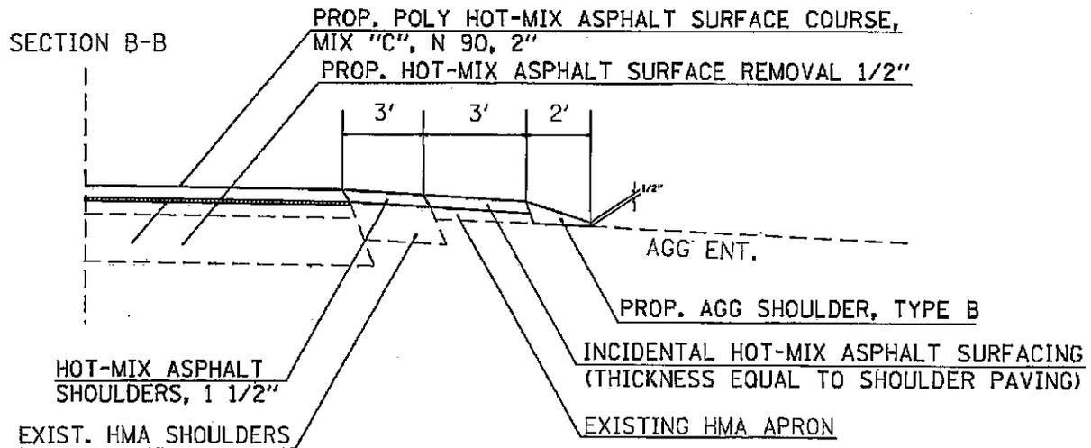
PREPARATION OF EXISTING SURFACE AND ANY EXCAVATION FOR ENTRANCES SHALL BE IN ACCORDANCE WITH ARTICLE 406.19 OF THE STANDARD SPECIFICATIONS.
