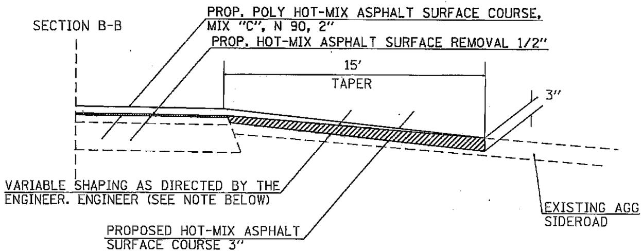
IF EXISTING SUB-BASE IS INADEQUATE, AS DETERMINED BY THE ENGINEER, THE SIDEROADS SHALL BE CORED OUT AND AGGREGATE SUB-BASE, TYPE B SHALL BE PLACED FOR BASE. THE COST OF CORING OUT THE SIDEROAD SHALL BE INCLUDED IN THE COST OF THE AGGREGATE BASE COURSE. IF EXISTING SUB-BASE IS DETERMINED TO BE ADEQUATE, THE AGGREGATE BASE COURSE SHALL BE DELETED AND THE PREPARATION OF THE BASE SHALL BE CONSTRUCTED ACCORDING TO ARTICLE 406.19
