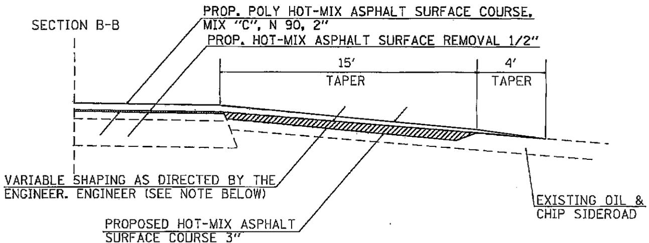
IF EXISTING SUB-BASE IS INADEQUATE, AS DETERMINED BY THE ENGINEER, THE SIDEROADS SHALL BE CORED OUT AND AGGREGATE SUB-BASE, TYPE B SHALL BE PLACED FOR BASE. THE COST OF CORING OUT THE SIDEROAD SHALL BE INCLUDED IN THE COST OF THE AGGREGATE BASE COURSE. IF EXISTING SUB-BASE IS DETERMINED TO BE ADEQUATE, THE AGGREGATE BASE COURSE SHALL BE DELETED AND THE PREPARATION OF THE BASE SHALL BE CONSTRUCTED ACCORDING TO ARTICLE 406.19
