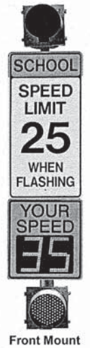
SOLAR-POWERED FLASHING BEACON ASSEMBLY N.T.S.
