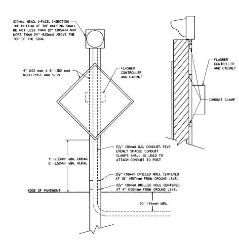
POST MOUNTED FLASHING BEACON WITH CONTROLLER AND CABINET
