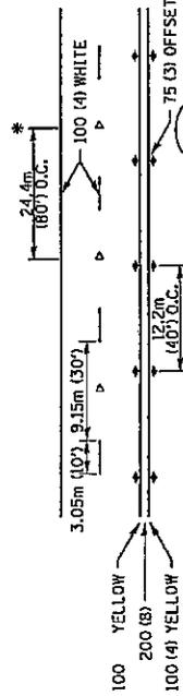
\* REDUCE TO 12.2m (40') O.C. ON CURVES WHERE ADVISORY SPEEDS ARE 15km/h (10MPH) LOWER THAN POSTED SPEEDS.
