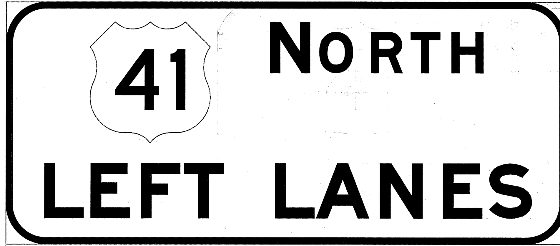
Structure No. 1S0161094L030.8-000 (RS-10) PL; 12.0" Radius, 2.0" Border, White on Green; [NORTH] ClearviewHwy-5-W; [LEFT LANES] ClearviewHwy-5-W specified length;
