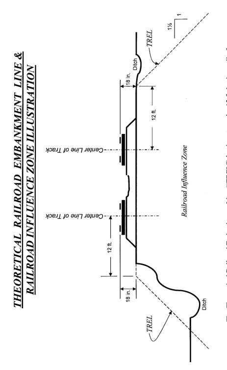
The Theoretical Railroad Embankment Line ("TREL") begins at a point 12 ft. horizontally from center line of track, 18 in. below top-of-rail, and extends downward on a 1½ (H) to 1(V) slope.
