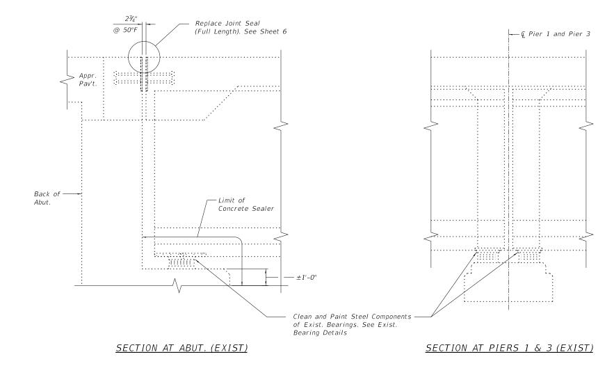
All existing bearings shall be cleaned according to SSPC-SP 11: Power Tool Cleaning to Bare Metal.
