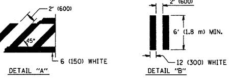
TYPICAL CROSSWALK MARKING
