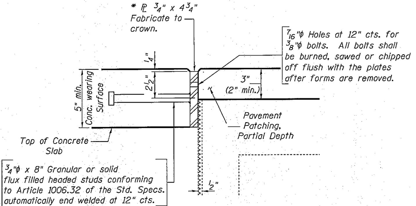
\* Furnish in segments of 20 ft. maximum length. Maximum space between installed segments shall be  $\frac{3}{16}''$ . Seal space with Silicone Sealant suitable for Structural Steel.
