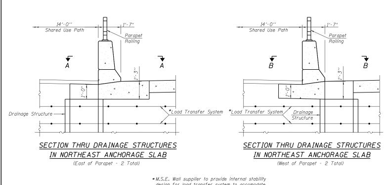
\*M.S.E. Wall supplier to provide internal stability design for load transfer system to accommodate drainage structures and pipes.
