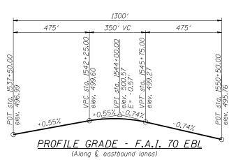
The profile grades depict the final elevations after grinding. Up to  $\frac{1}{4}$ " will be ground off the bridge decks and approach slabs.
