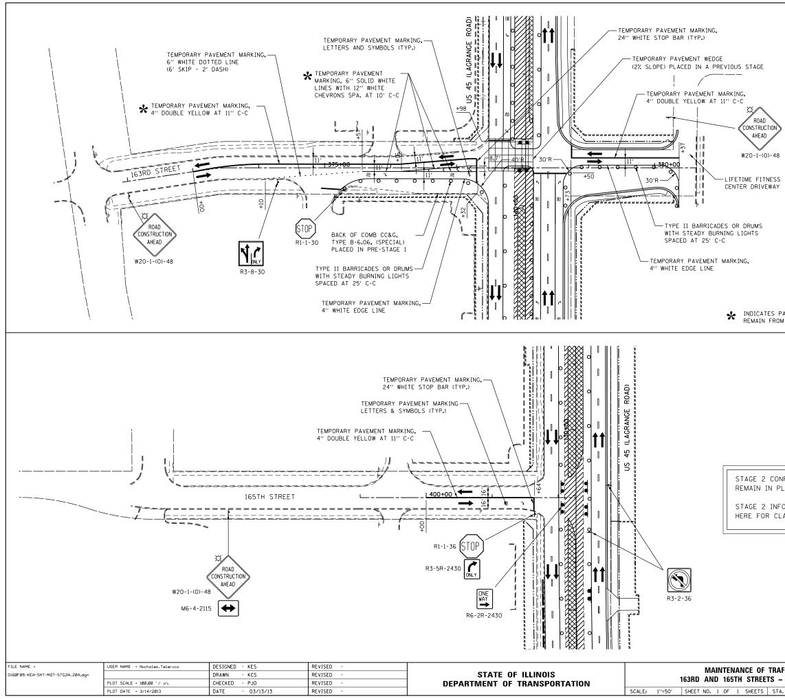
✤ INDICATES PAVEMENT MARKING TO REMAIN FROM PREVIOUS STAGE
