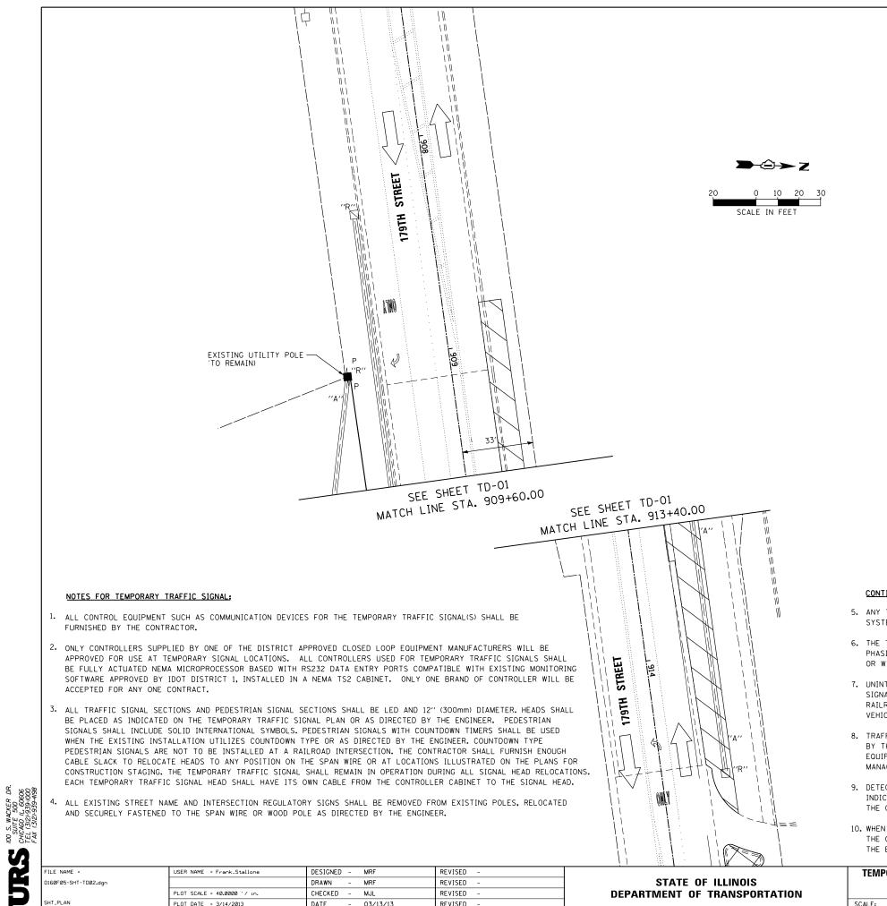
5. ANY TEMPORARY SIGNAL WITHIN AN EXISTING CLOSED LOOP TRAFFIC SIGNAL SYSTEM SHALL BE INTERCONNECTED TO THAT SYSTEM USING SIMILAR BRAND CONTROL EQUIPMENT.
