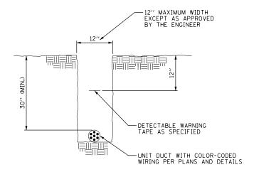
TYPICAL UNIT DUCT IN TRENCH DETAIL
