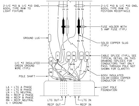
TYPICAL POLE BASE WIRING DETAIL
