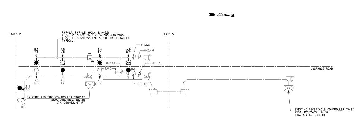
EXISTING LIGHTING CONTROLLERS "RWP-1" & "H-2" STAGE 3 WIRING MODIFICATION DIAGRAM N.T.S. (NOTES 2, 3, 4)
