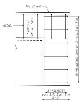
TYPICAL END CAP DETAIL (v160(E) bars in F.F. not shown for clarity)
