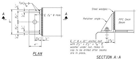
Cost of retainer and accessories are included with Precast Prestressed Concrete Deck Beams. Equivalent rolled angle with stiffeners will be allowed in lieu of welded plates.
