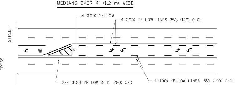
A MINIMUM OF TWO PAIRS OF TURN ARROWS SHALL BE USED, WHITE IN COLOR. ADDITIONAL PAIRS SHALL BE PLACED AT 200' (60 m) TO 300' (90 m) INTERVALS.
