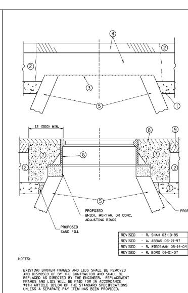
IF THE EXISTING LIDS ARE OPEN, THE FRAME WILL BE ADJUSTED TO THE ELEVATION OF THE MILLED PAVEMENT SURFACE PRIOR TO THE MILLING OPERATION. THE FRAME WILL NOT BE REMOVED AND COVERED BY THE METAL PLATE.
