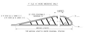
CANNOT BE ATTAINED, USE 5 (FIVE) EQUALLY SPACED DIAGONAL LINES.
