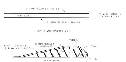
DIAGONAL LINE SPACING: 50' (15 m) C-C (LESS THAN 30MPH (50 km/h))
