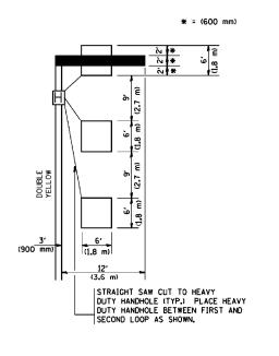
NOTE: DUAL LEFT TURNS NOT SHOWN REFER TO PLAN SHEET FOR DETECTOR LOOP REPLACEMENT
