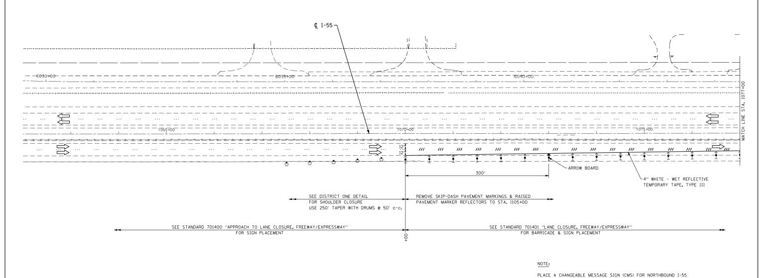
TRAFFIC 1000'± SOUTH OF CREST OF I-55 VERTICAL CURVE SOUTH OF BLUFF RD. CMS SHALL DISPLAY "WATCH FOR STOPPED TRAFFIC".
