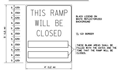
THESE SIGNS ARE REQUIRED ON BOTH SIDES OF THE RAMP, MINIMUM OF 1 WEEK IN ADVANCE OF THE CLOSURE.
