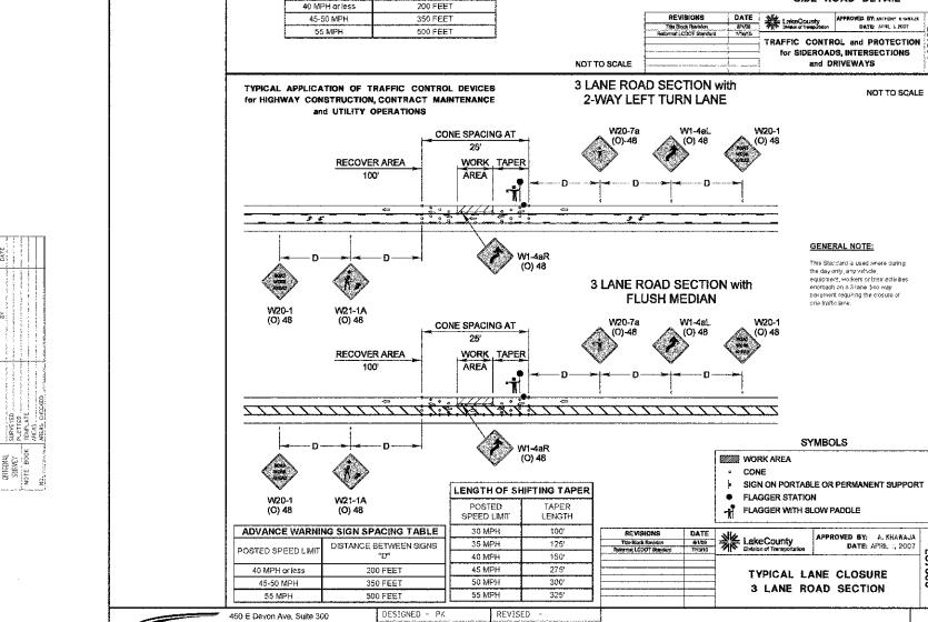
TYPICAL APPLICATION OF TRAFFIC CONTROL DEVICES for HIGHWAY CONSTRUCTION, CONTRACT MAINTENANCE and UTILITY OPERATIONS
