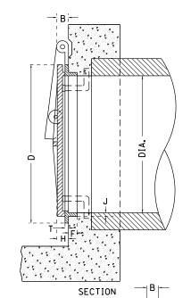
IT IS INTENTED THAT THE AUTOMATIC FLAP GATES SHALL BE A COMMERCIAL PRODUCT PRODUCED BY A RELIABLE MANUFACTURER. THE GATE MAY BE MADE OF CAST IRON, CAST STEEL OR OTHER SUITABLE MATERIALS. THE DESIGN MAY DIFFER FROM THE DRAWING IF IT WILL WORK IN A SATISFACTORY, TROUBLE FREE MANNER AND WILL WITHSTAND THE WATER PRESSURE AT THE INSTALLATION LOCATION. THE GATE SHALL BE APPROVED BY THE ENGINEER.
