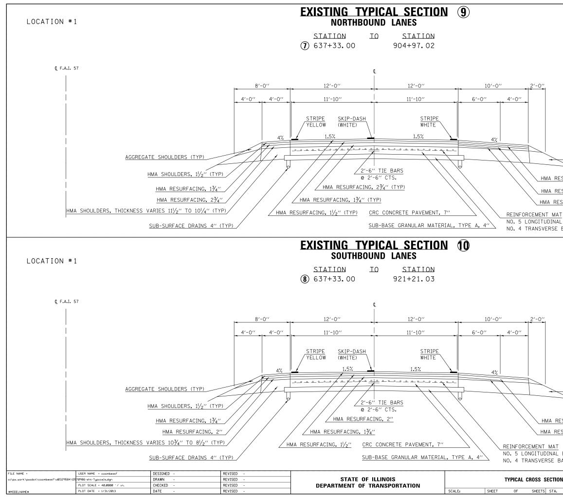
EMBANKMENT (TYP) HMA RESURFACING, 11/2" HMA RESURFACING, THICKNESS VARIES 11/4" TO 13/4" HMA RESURFACING, THICKNESS VARIES 13/4" TO 3/4"
