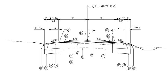
CONSTRUCT CUT SECTION AS SHOWN IN STATION CROSS SECTIONS
