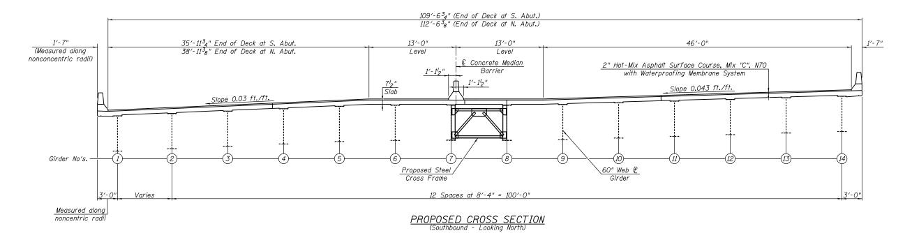
Note: All transverse dimensions are measured along the radii of F.A.I. Rt. 255 curves except as noted.
