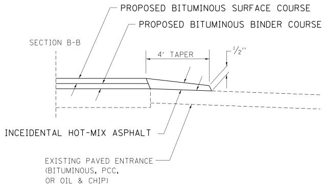
PREPARATION OF EXISTING SURFACE AND ANY EXCAVATION FOR ENTRANCES SHALL BE IN ACCORDANCE WITH ARTICLE 406.09 OF THE STANDARD OF SPECIFICATIONS.
