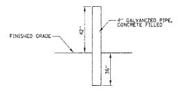
NOTE: BOLLARDS SHALL BE INSTALLED 6' CENTER TO CENTER
