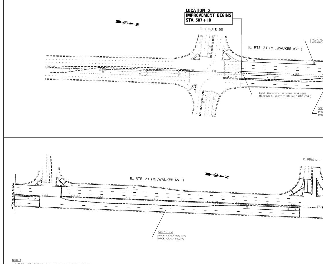
ALL CRACK AND JOINT SEALING SHALL BE DONE AT ALL PAVEMENT JOINT EXECPT ON LOCATIONS WHERE THE GUTTER HAS BEEN OVERLAID
