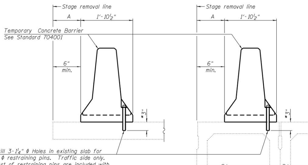
Drill 3-1/4"  $\phi$  Holes in existing slab for 1"  $\phi$  restraining pins. Traffic side only. Cast of restraining pins are included with Temporary Concrete Barrier. No restraint is required when "A" is greater than 3'-1".
