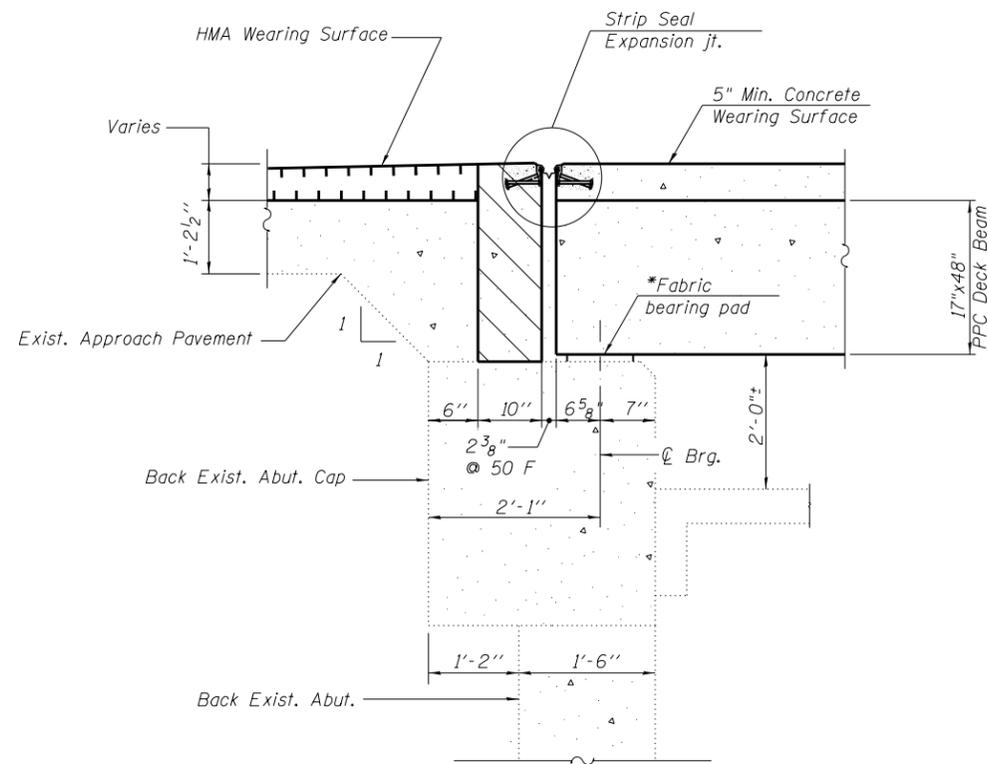
**SECTION THRU EXISTING ABUTMENTS**
