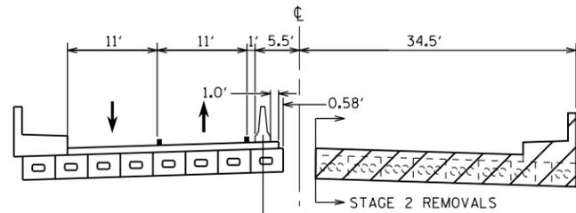
TEMPORARY CONCRETE BARRIER (ANCHORED)
