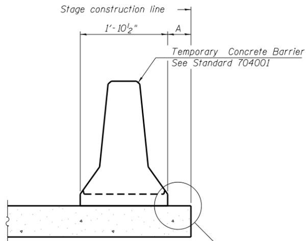
When "A" is 3'-1" or less, the temporary concrete barrier shall be restrained to the new slab according to Detail I, II or III. No restraint is required when "A" is greater than 3'-1".
