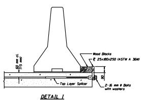
The 25x180x250 Plate shall not be removed until Stage II Construction forms and reinforcement bars are in place.
