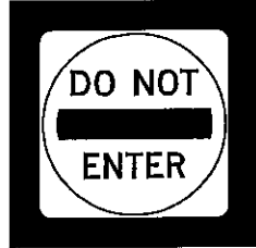
(E) 48" X 48" Std. 36" X 36" R5-1 or 36" X 36" overall with Std 36" X 36" R5-1 where noted
