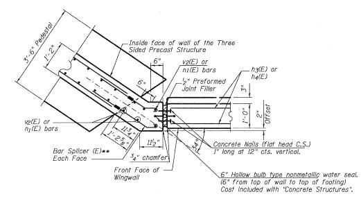
\*\* Bend Bar Splicer (E) in field. Cost included with "Three-Sided Precast Concrete Structures, 28'x10'". <u>DETAIL B</u>
