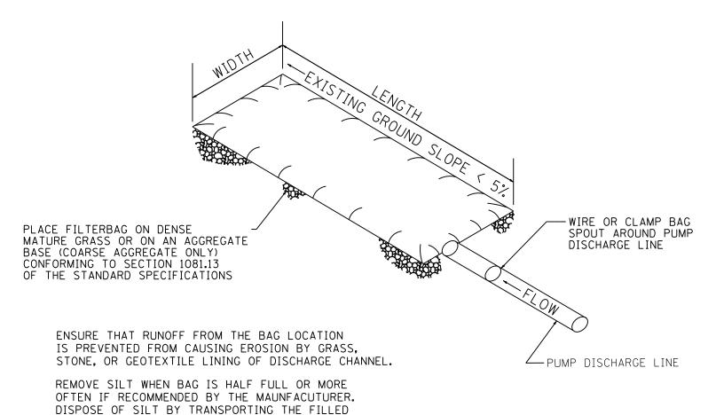
BAG TO DISPOSAL AREA. SLIT THE BAG, BLEND SILT INTO EXISTING TOPOGRAPHY, SEED AND MULCH MAINTAIN EXTRA FILTER BAGS ON SITE.
