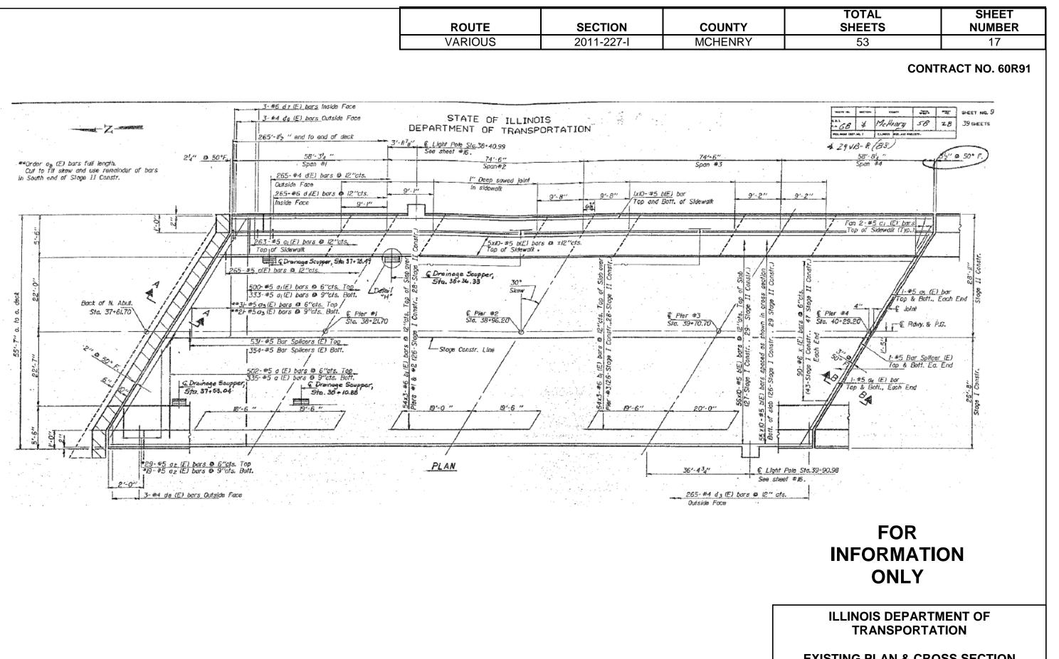
**EXISTING PLAN & CROSS SECTION** LOCATION 1 (SN 056-0007) **US 14 OVER RR AND MCCOOB ST** SHEET 1 OF 4
