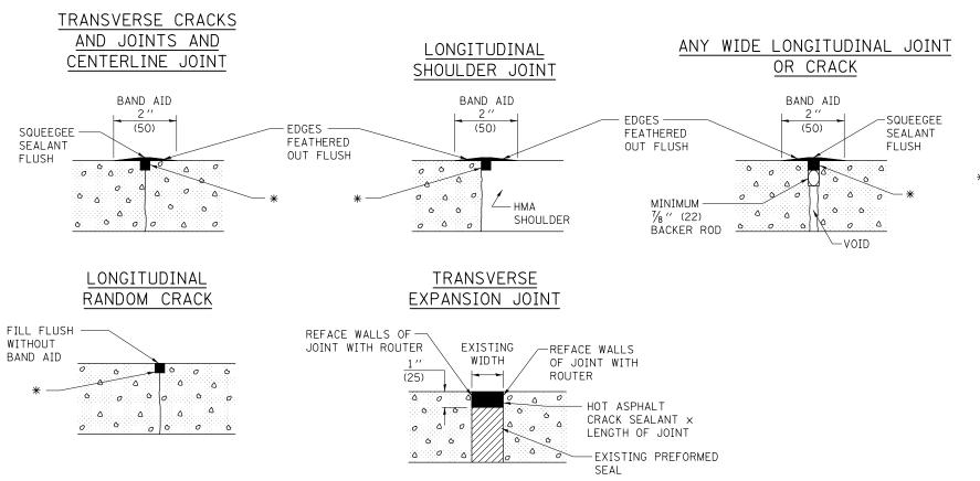
\* HOT ASPHALT CRACK SEALANT APPROX. 3/4 " × 3/4" × LENGTH OF CRACK. ACTUAL QUANTITY WILL VARY AS NEEDED FOR PRIMARY OR SECONDARY WORKING CRACK.
