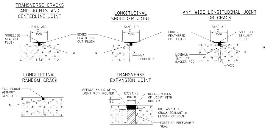
\* HOT ASPHALT CRACK SEALANT
