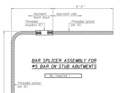
FILE NAME USER NAME = steffenmk DESIGNED - KLB REVISED BAR SPLICER ASSEMBLY AND M STATE OF ILLINOIS c:\pw\_work\pwidot\steffenmk\d0270599 74536-sht-brdetails-0960039.don DRAWN KLB REVISED STRUCTURE N PLOT SCALE = 40.0000 '/ in. CHECKED MEA REVISED **DEPARTMENT OF TRANSPORTATION** SCALE: SHEET NO. 8 OF 9 SHEETS PLOT DATE = 1/25/2012 DATE 10/31/11 REVISED
