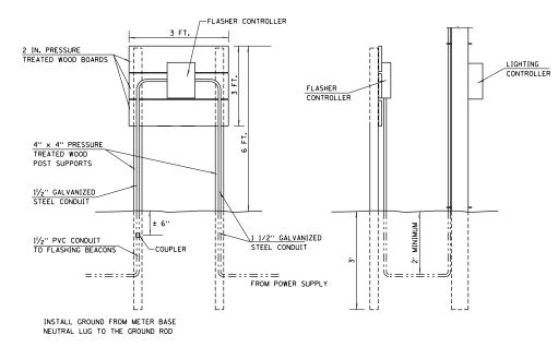
THIS DETAIL SHALL BE USED IN CONJUNCTION WITH STANDARD 805001 ELECTRIC SERVICE INSTALLATION. SPECIAL
