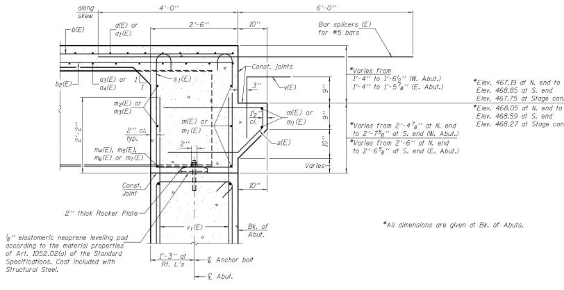
SECTION A-A Dimensions at right angles to abutment, except as shown.
