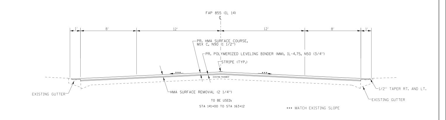
NOTE: HMA REMOVAL IN GUTTER AREAS SHALL BE INCLUDED IN HMA SURFACE REMOVAL, 2 1/4"
