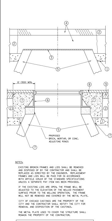
WHEN STRUCTURES ARE TO BE ADJUSTED OR RECONSTRUCTED, THE LOWERING AND RAISING OF THE FRAMES AND LIDS WILL NOT BE PAID FOR SEPARATELY BUT WILL BE INCLUDED IN THE COST OF THE CORRESPONDING PAY ITEM.
